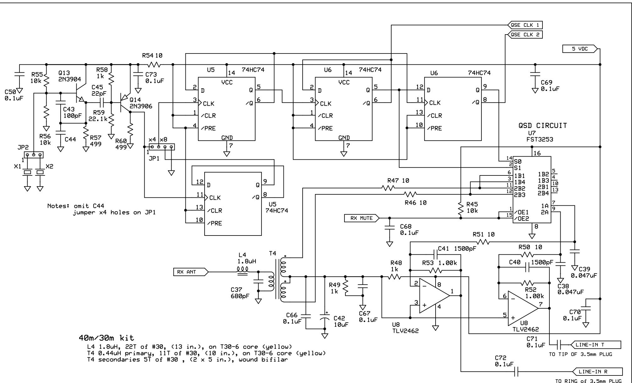
Note: Components mounted to the bottom of the board include size 1206 SMT capacitors C50 through C73 and SOICs U1, U2, U3, U5, U6, U7 and U8
