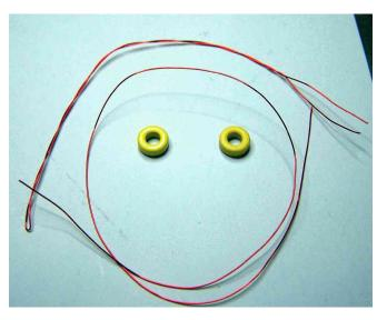
The smiley-face picture shows two T25-6 cores, the wire for the primary winding, and the twisted bifilar wire "hair[in" for the secondary winding.
