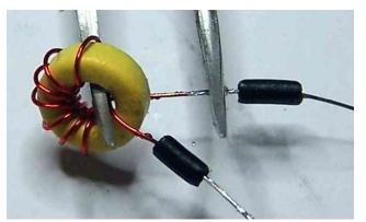
One easy way to remove the insulation and tin the leads is to slather flux paste on the leads and then draw the leads through a fresh blob of solder on a hot iron. The flux acts to helop remove the debris from the enamel insulation. A couple of passes through the flux/solder cycle and the leads come out nicely tinned (the picture suggests the leads might need another pass through the flux/solder cycle).
