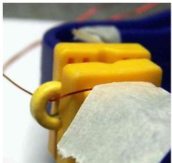
picture. Do not put too much pressure on the toroid when clamping it, since these powdered iron cores can crumble under too much pressure. This is unlikely if you are using softjawed clamps like the Irwin. The builder begins the winding with the first of the eight turns. Remember, any pass through the "doughnut hole" counts as a single turn. This picture shows a single turn.
