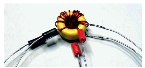
Tinning the leads is accomplished as described with the primary. You will need to identify and mark one of the two pairs of secondary leads. This is best done using an ohmmeter to identify continuity.
