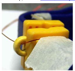
picture. Do not put too much pressure on the toroid when clamping it, since these powdered iron cores can crumble under too much pressure. This is unl
